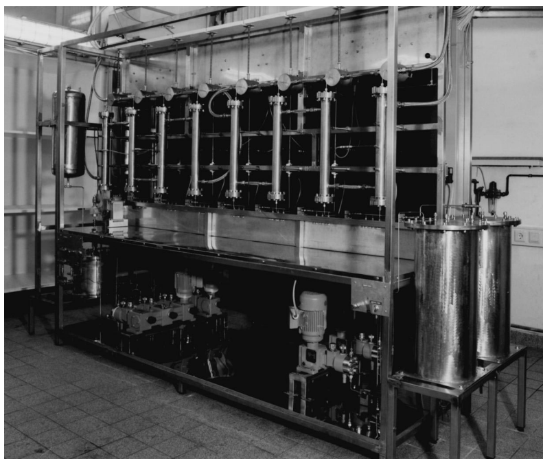
Fig. 2. Photo of the SMB plant (without insulation).
